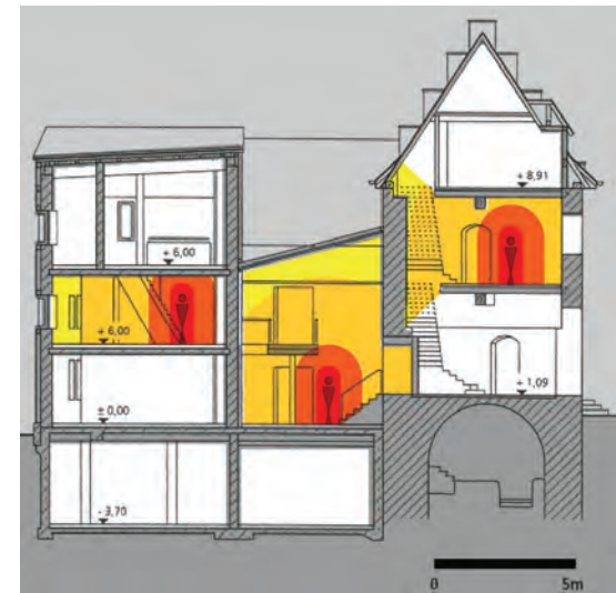
Figure 3-35 Section A of the Korbach museum shows the new concrete addition, the covered access, and the historical house with an underground geological exhibit.
