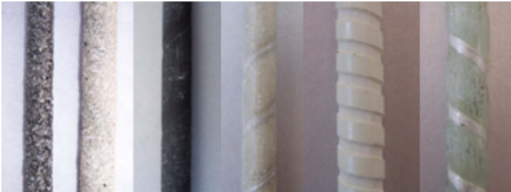
Figure 2.2: Various FRP Surface Treatments (Baena et al., 2009)
