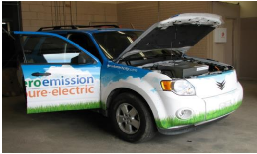
Figure 4-1 Converted Ford Escape (EV-ACX2.5)
