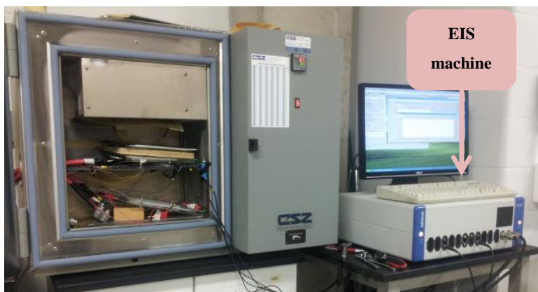
Figure 3-19: Experimental setup for the EIS test.
