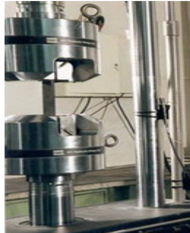
Figure 4.9. The experimental setup for material fatigue testing.
