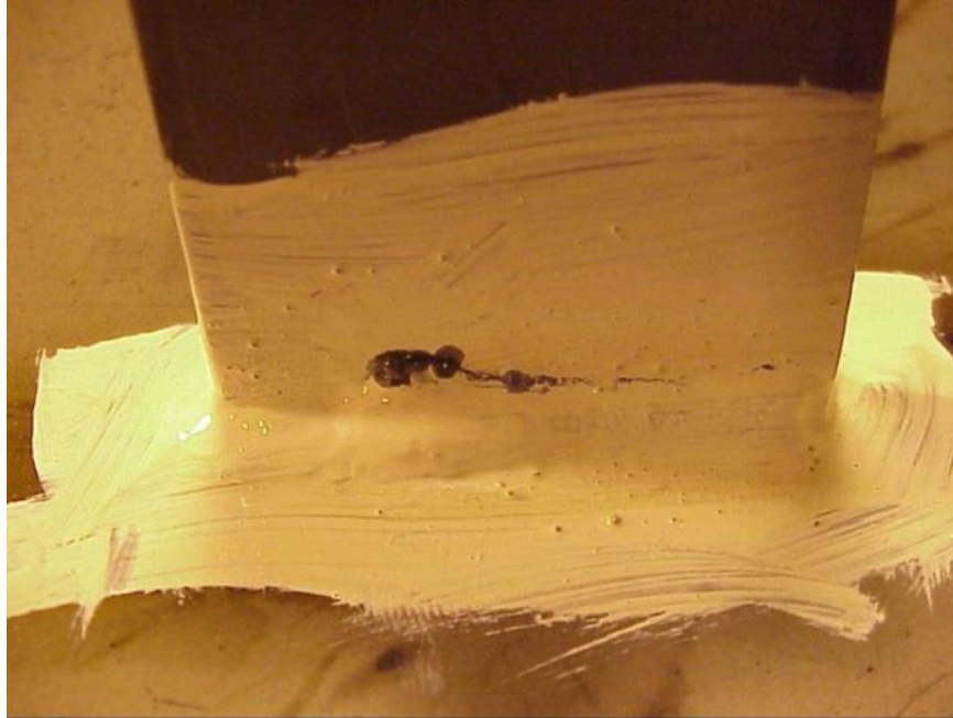
Figure 5-21: Fatigue location of fatigue cracks in the vertical attachment; gusset weld joint with symmetric welds ( F=468 N). Cracks located in the region of predicted maximum stress
