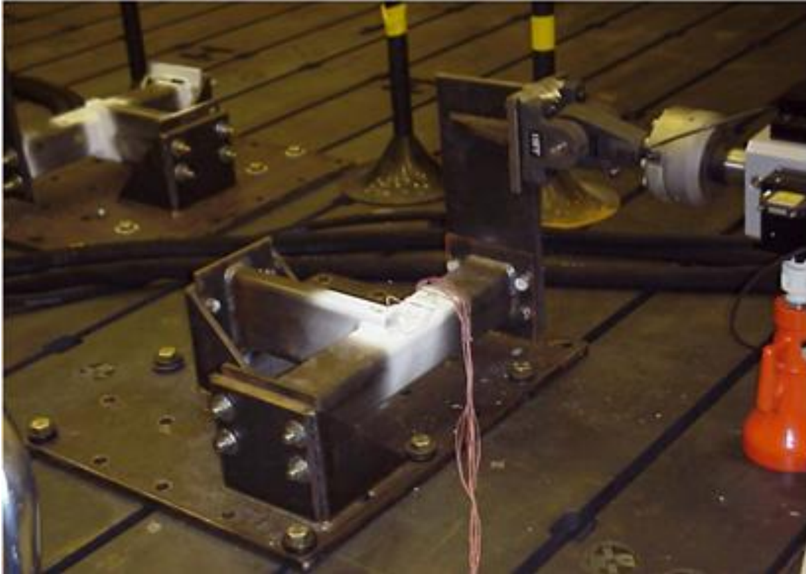
Figure 5-39: The fatigue test setup arrangement – tubular weldment
