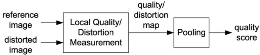
Figure 2.8: Two stage structure of image quality assessment systems. Figure obtained from [90].
