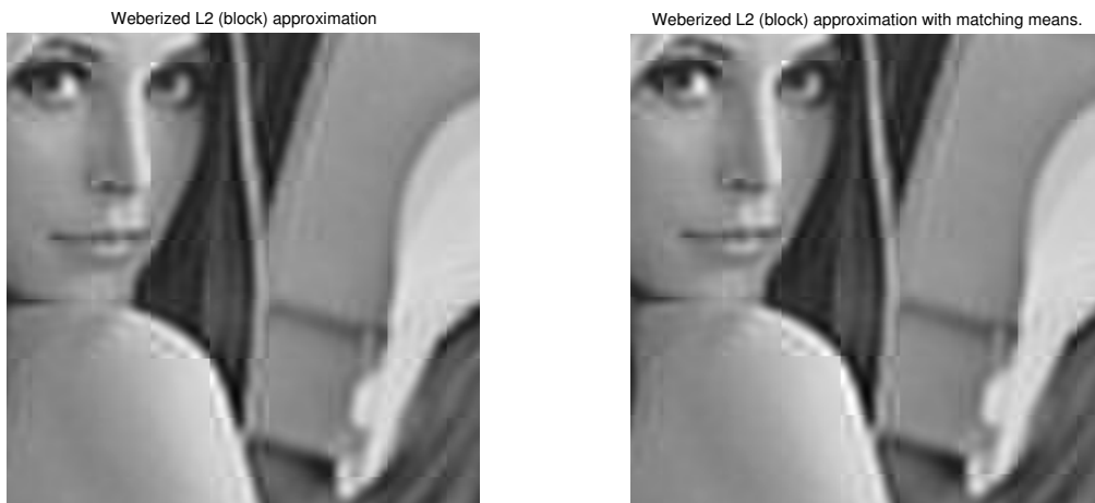
Figure 6.8: “Weberized” L^2 (left) and “Weberized” L^2 with matching of means (right) approximations to Lena image using N = 43 2D DCT basis functions over 32 \times 32 -pixel blocks comprising the shoulder region of Lena image (magnified). Original size of images: 512 \times 512 pixels.
