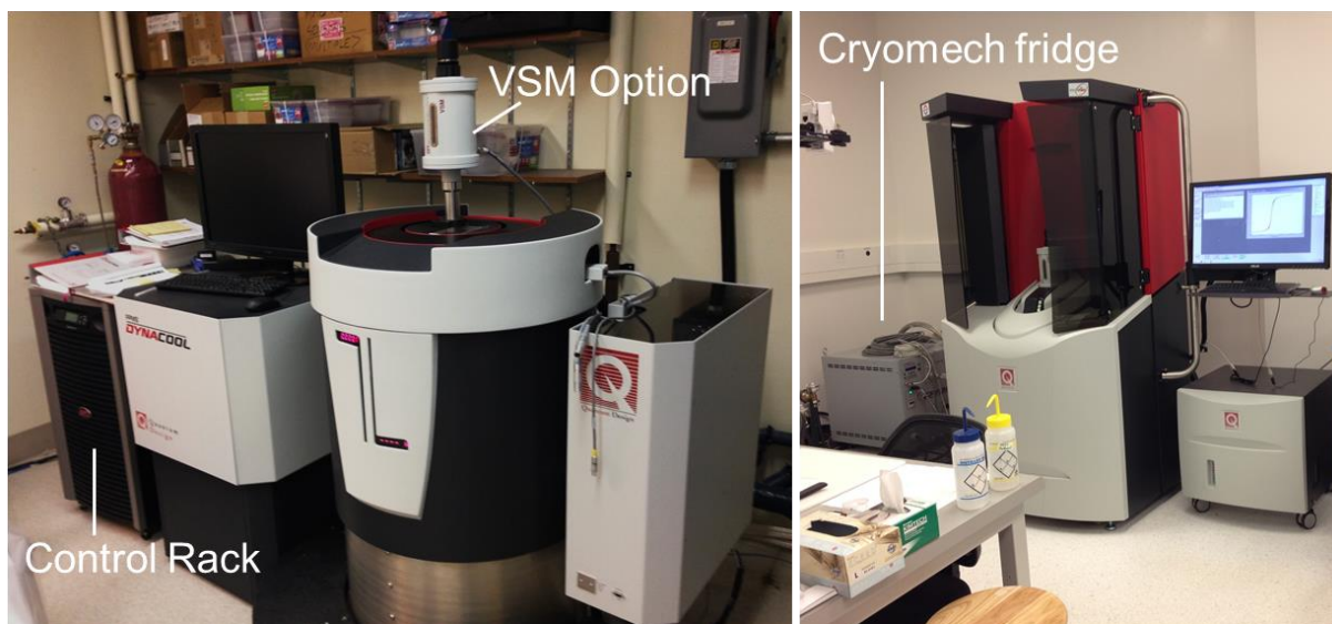
Figure 2.8 (a) Photograph of the computer, pump cabinet and cryostat of the Quantum Design Dynacool physical property measurement system. (b) General setup for Superconducting Quantum Interference Device (SQUID) for magnetic properties measurements for hybrid NPs by Quantum Design Magnetic Property Measurement System (MPMS)-VSM system.
