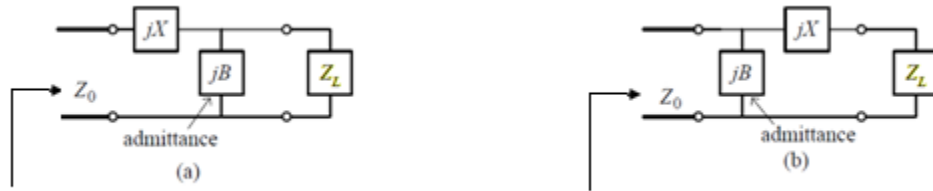
Figure 4.2: L-topology impedance matching networks. (a) z_L inside the 1+jx circle and (b) z_L outside the 1+jx circle
