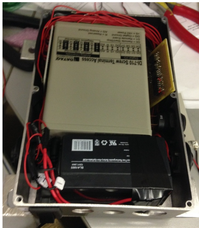
Figure 23 - Smart Tire Monitoring System with DI-710 DAQ
