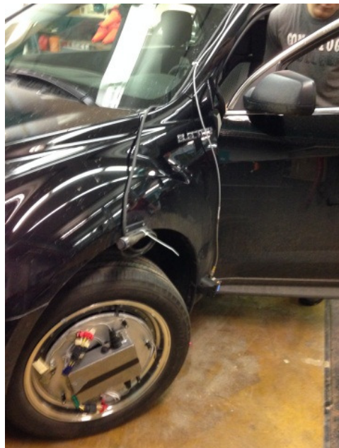
Figure 25 - Fully Assembled Smart Tire Monitoring System Installed on Chevrolet Equinox EV
