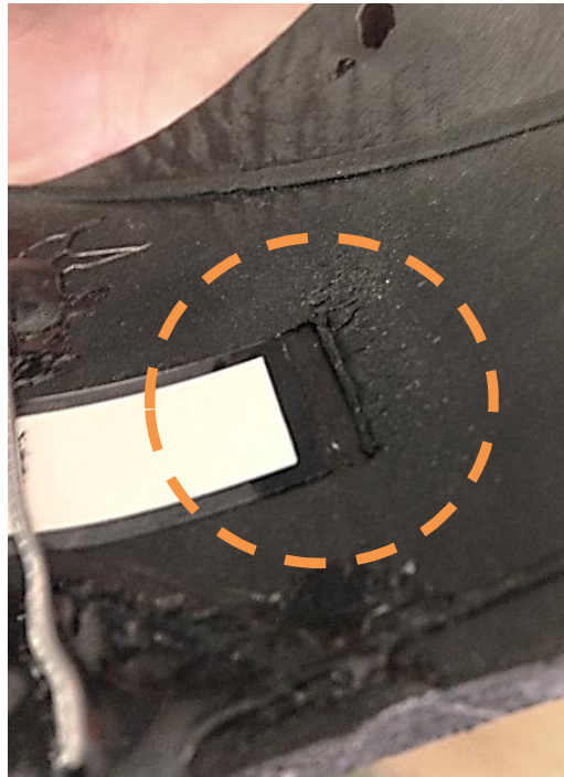
Figure 15 - PVDF Sensor Creating a Dent into the Rubber Specimen
