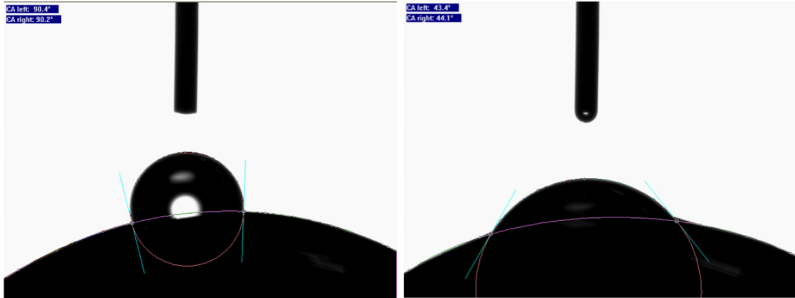
Figure 1-11: Advancing contact angles on relatively non-wettable (left) and wettable (right) contact lenses.
