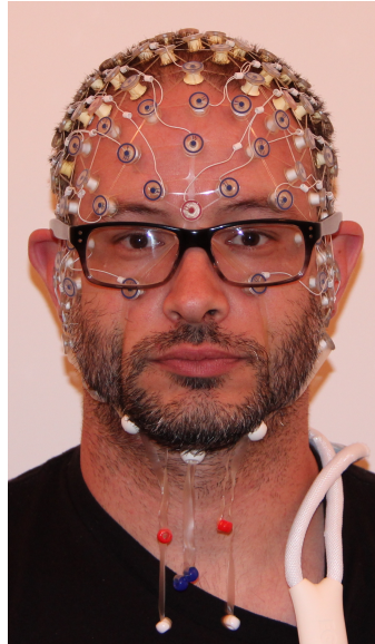
Figure 1.8: A modern EEG cap with 128 electrodes. Electrodes come as far down the head as reasonable to try and pick up the activity originating from the bottom of the brain. There are electrodes directly above and below each eye, which can be used to isolate activity due to eye movements.
