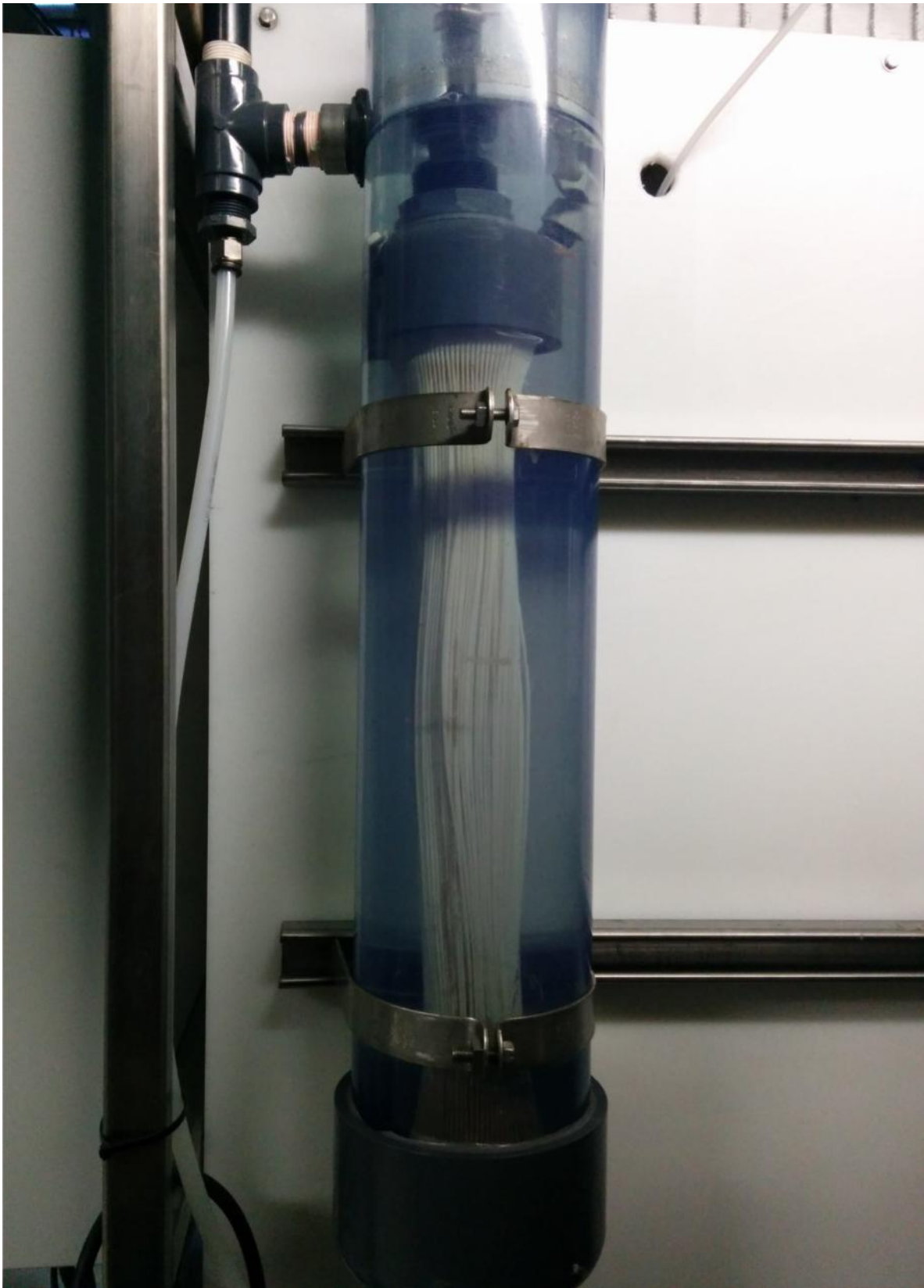
Figure A-6. Pilot#2 ZeeWeed500 ® membrane module at the beginning of operation
