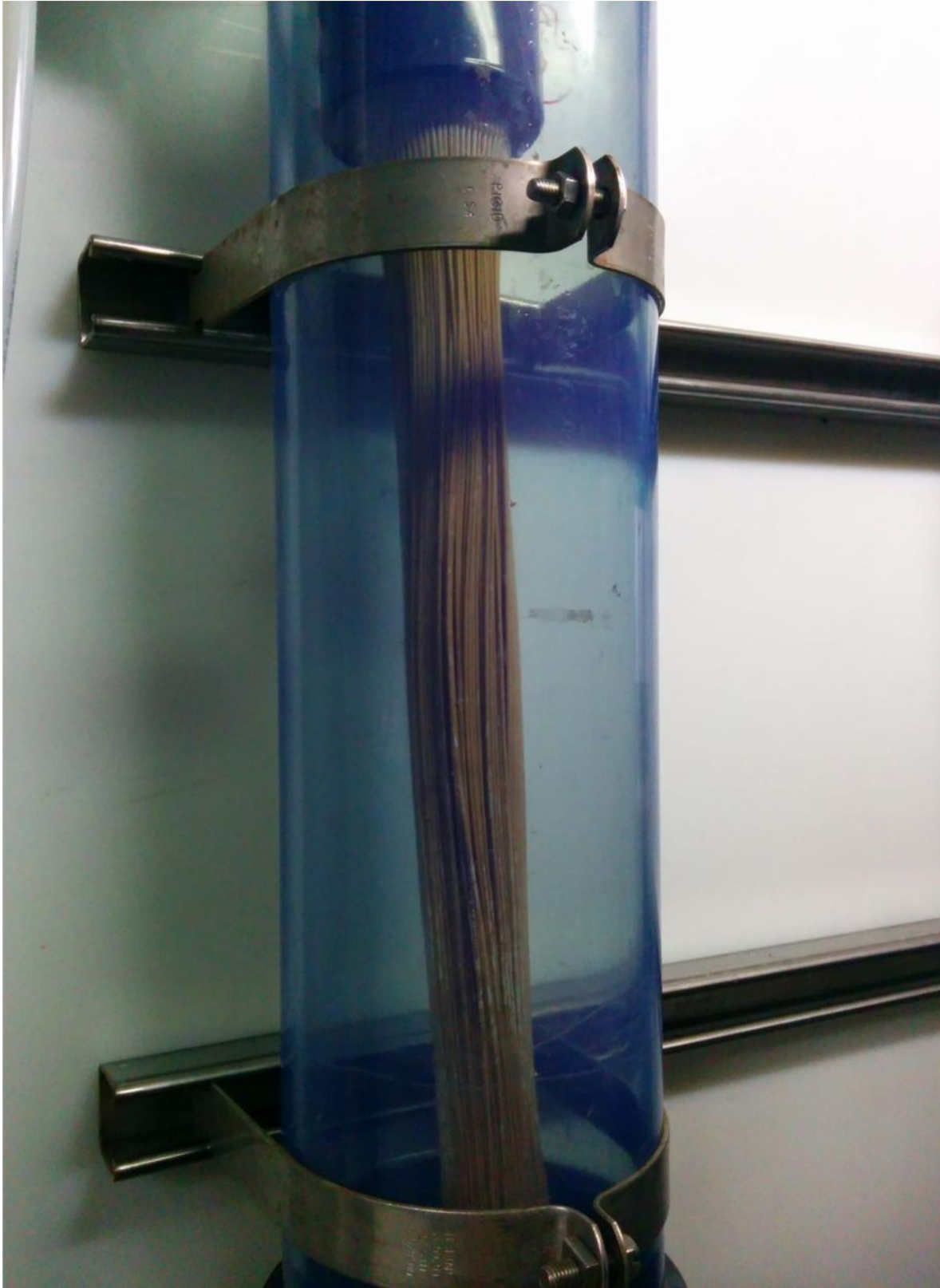
Figure A-7. Fouled Pilot#2 ZeeWeed500 ® membrane module during operation before recovery cleaning
