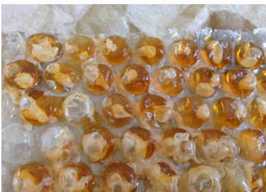
2-39 Bubble wrap injected with alkalized alginate. (By the author, 2013)
