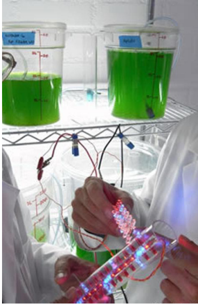
3-02 OriginOil's Biofeedback System is an active monitoring system specifically designed for algae bioreactors. It adjusts conditions such as lighting and pH to maintain the health of the culture. (OriginOil, 2012)
