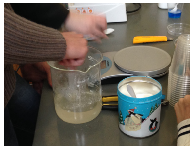
2-37 Mixing sodium hydroxide and alginate into hot water. (By the author, 2013)
