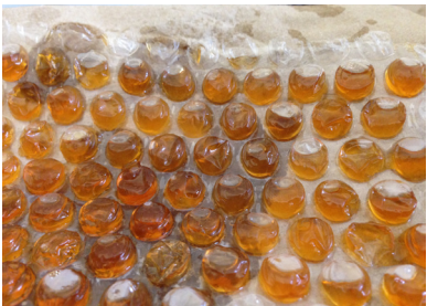
2-39 Bubble wrap injected with alkalized alginate. (By the author, 2013)
