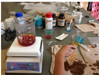
2-38 Hot plate of alginate and its injection into bubble wrap with a syringe and needle.
