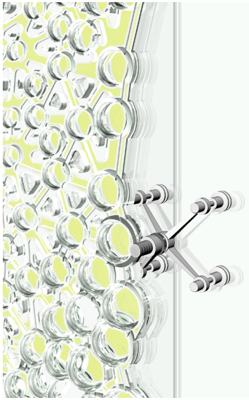
How the embedded hooks in the textile would pin to a spider glass connector.
