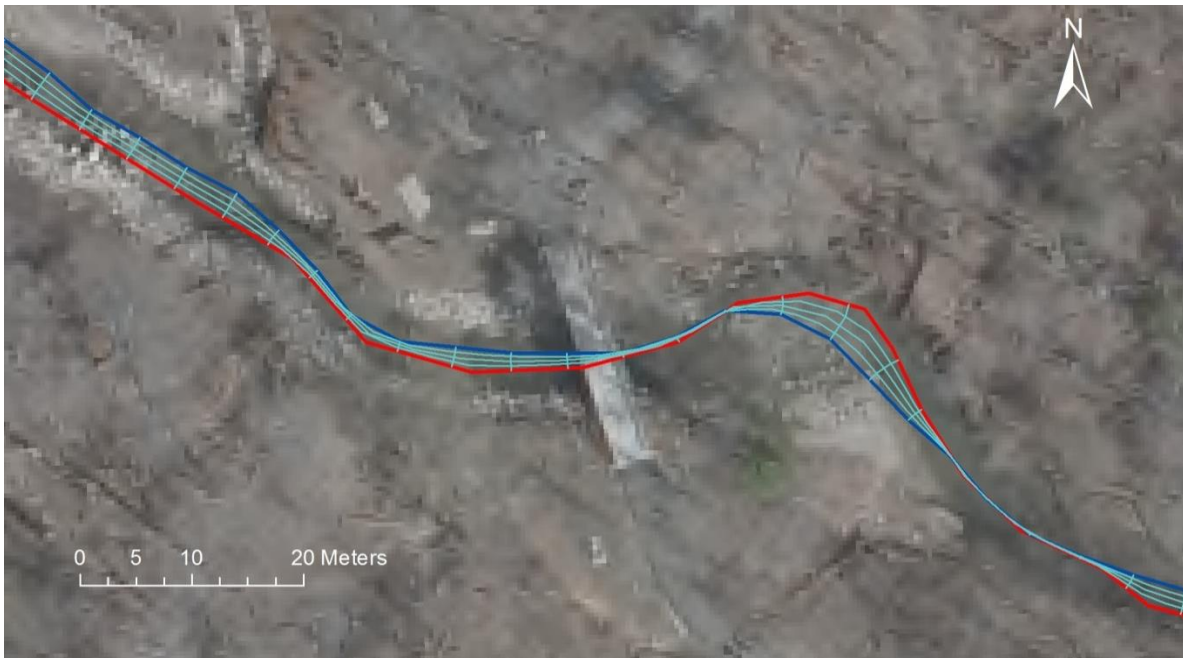
Figure 7. Channel Planform Statistics Tool output showing lateral movement from the blue reference line (2009) to the red line (2012). Lateral measurements to the right of the reference line are positive and negative to the left.
