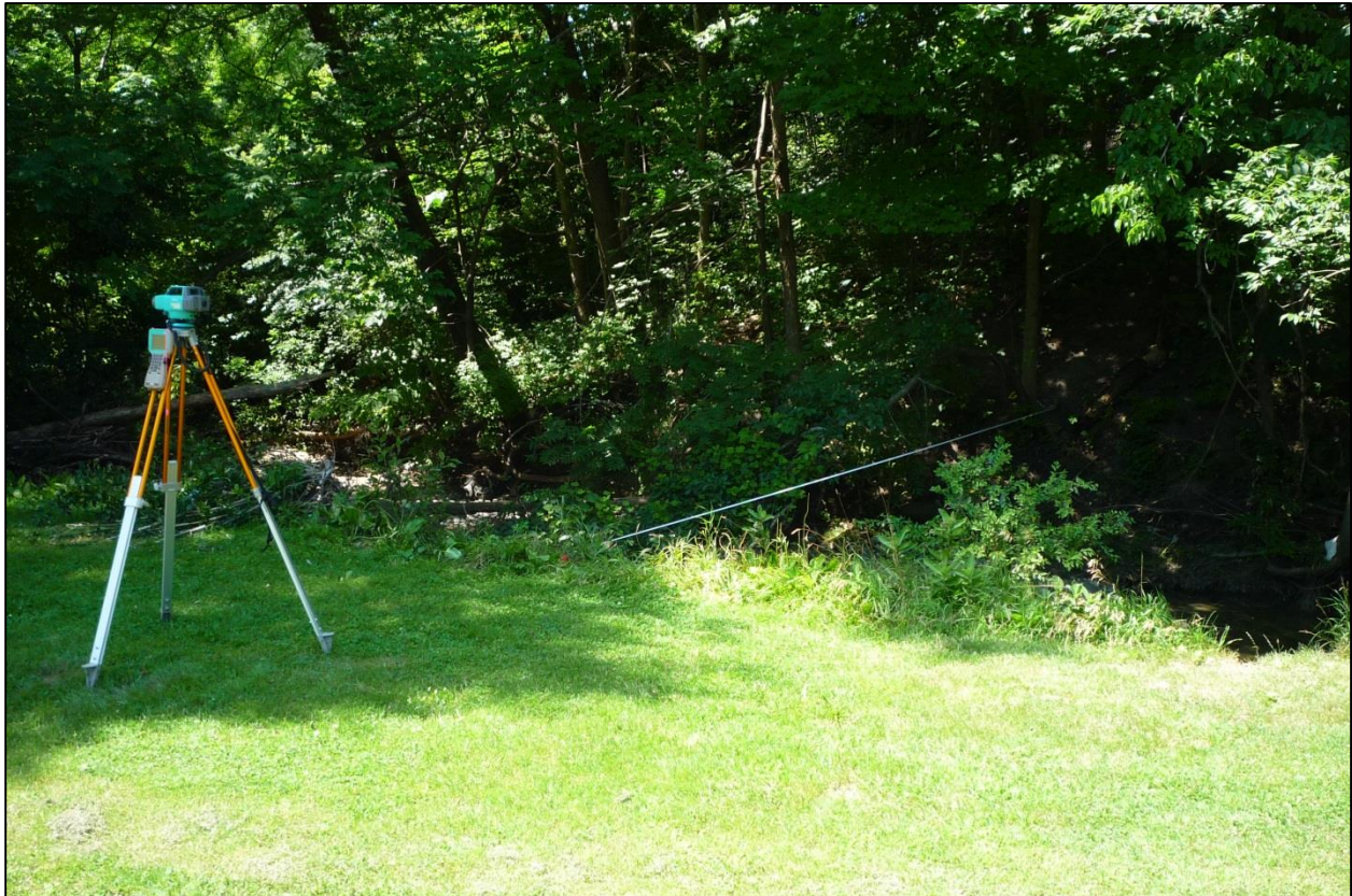
Figure 8. Auto level configuration for surveying cross sections.
