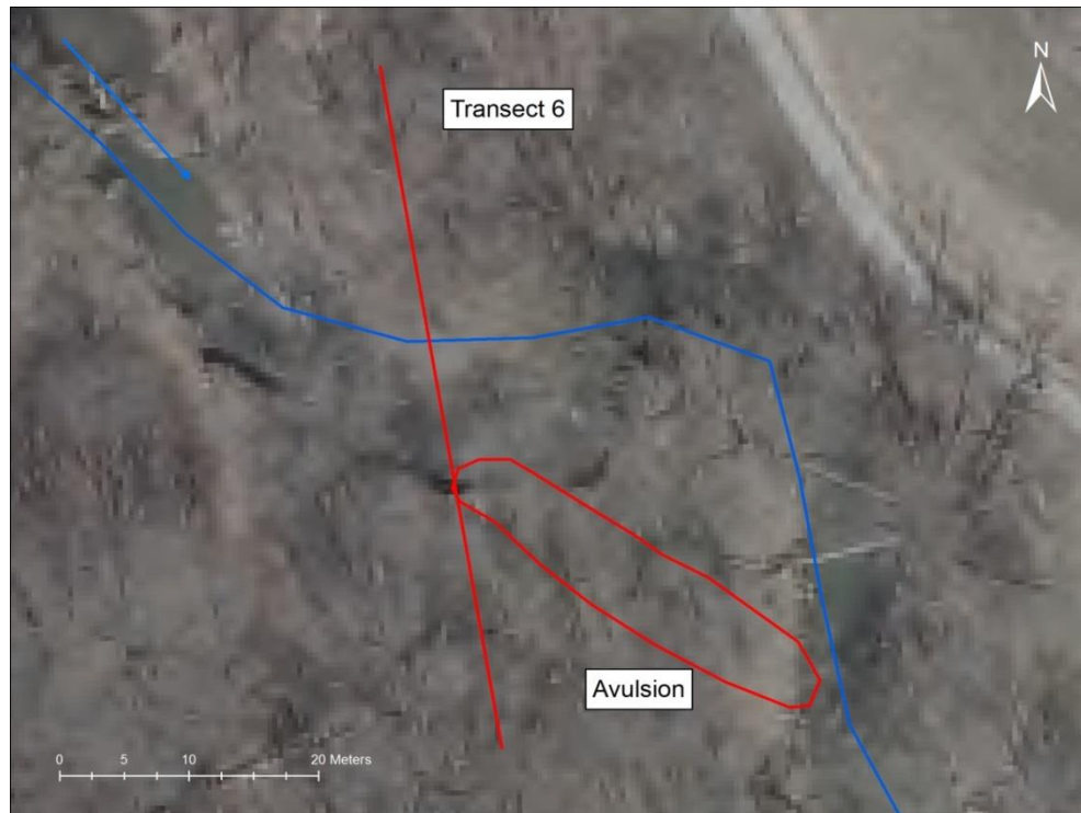
Figure 68. Active avulsion located near Transect 6 in Section 2 with headcut propagating upstream.
