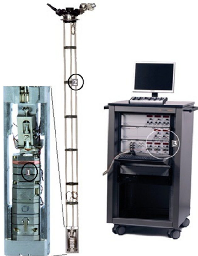
Figure 2.13. Cryogenic Atomic Force Microscope from Attocube. 1. AFM Stand with the ferrule, 2. AFM stick that already holds the AFM stand in 1, 3. AFM Controller Electronics. [55]
