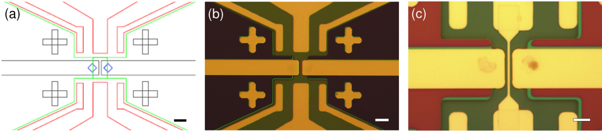
Figure 3.1: a) The photomask patterns used for CNT device fabrication, where the scale bar is 10\ \mu\text{m} . b) A device with source-drain contacts, trench etching, and gate pads, where the scale bar is 10\ \mu\text{m} . c) A finished device, after CVD growth, showing the EBL-defined fine gate and photolithography-defined catalyst islands, where the scale bar is 5\ \mu\text{m} .
