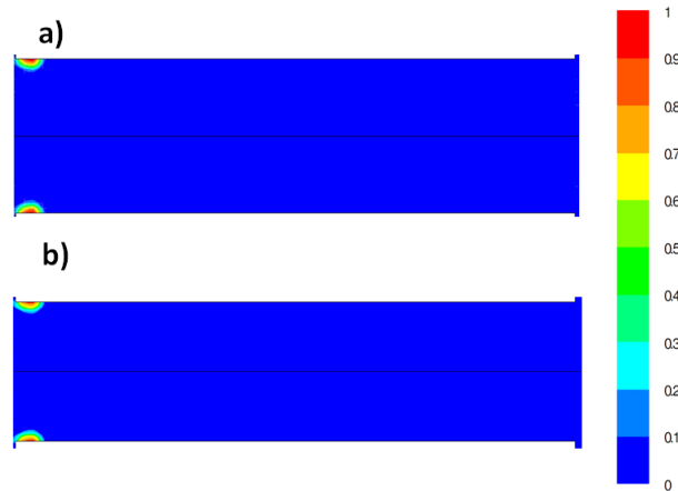
Figure 5.15: Vapour volume fraction contours for a) smooth wall and b) wall roughness height of 5 microns for diesel at inlet pressure of 15 MPa and outlet pressure of 5 MPa
