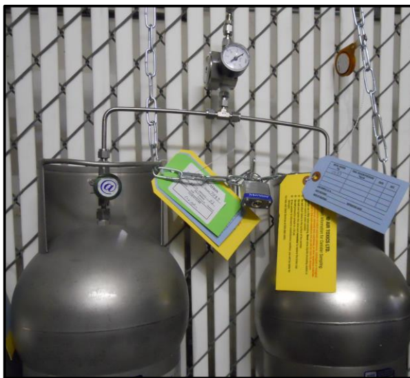
Figure 1-11: Photo of two 6L Summa canisters and a 3M OVM 3500 sampler (upper right)
