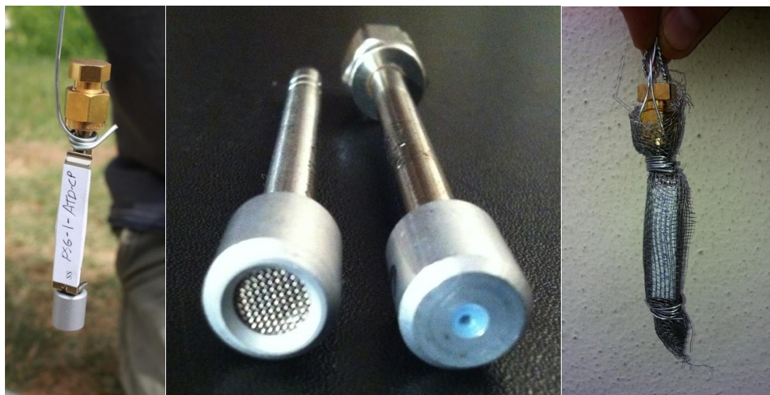
Figure 1-10: ATD tube sampler, regular and low-uptake rate caps, and protective mesh
