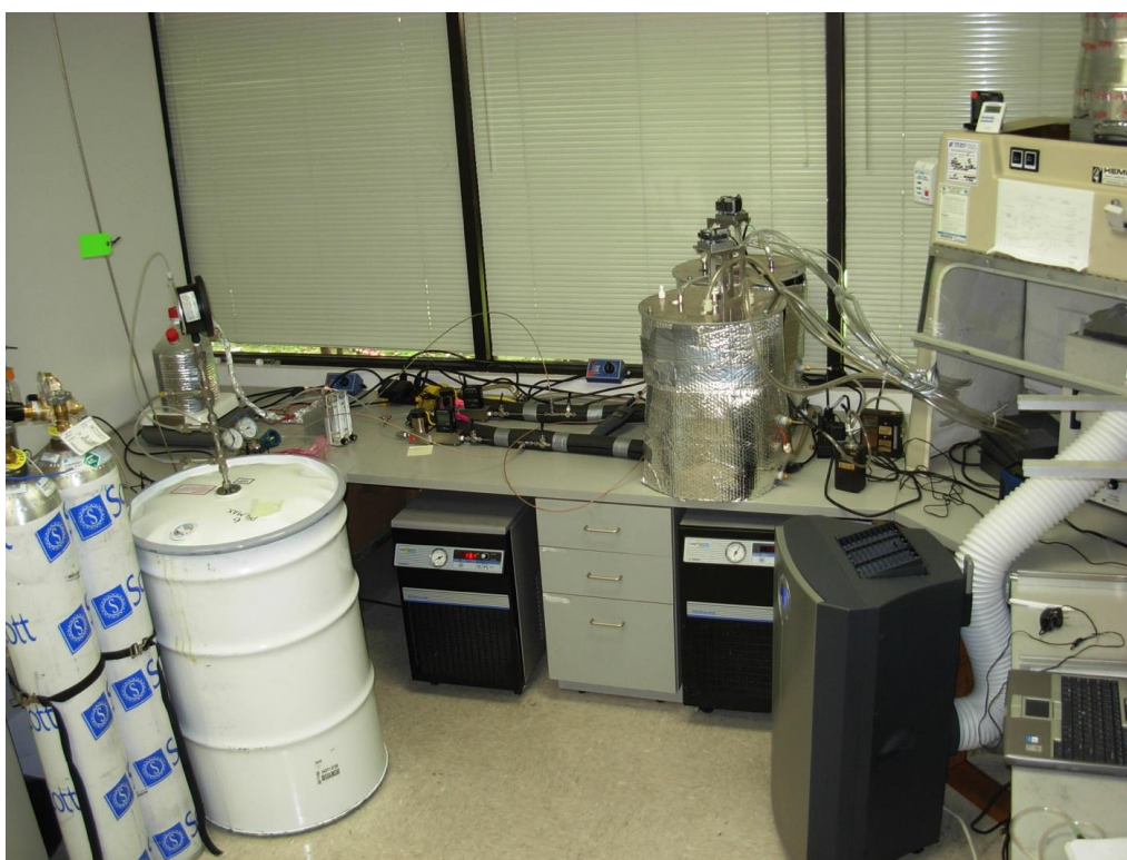
Figure 3-3: Low concentration test apparatus, including (left to right): compressed gas cylinders containing 10 VOCs, drum of activated carbon for purifying dilution air, humidification vessel, mass flow controllers, exposure chambers (covered with insulation), constant temperature bath, and discharge lines to fumehood (photo courtesy of Air Toxics Ltd.)
