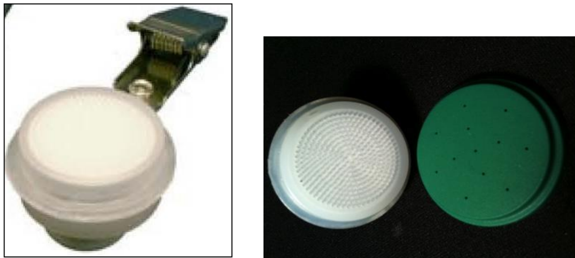
Figure 1-6: SKC Ultra sampler with regular (white) and low-uptake cap (green) (image at left courtesy of SKC)
