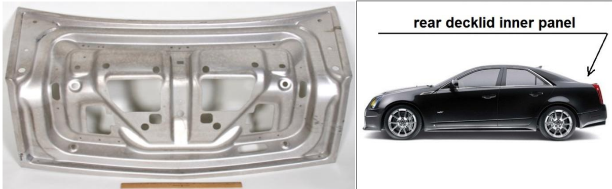
Figure 1.3: a) Experimental decklid inner panel formed by hot gas blow-forming process on AZ31B (Min et al., 2012b), b) GM's Cadillac CTS (Photo: Hogan, 2008).
