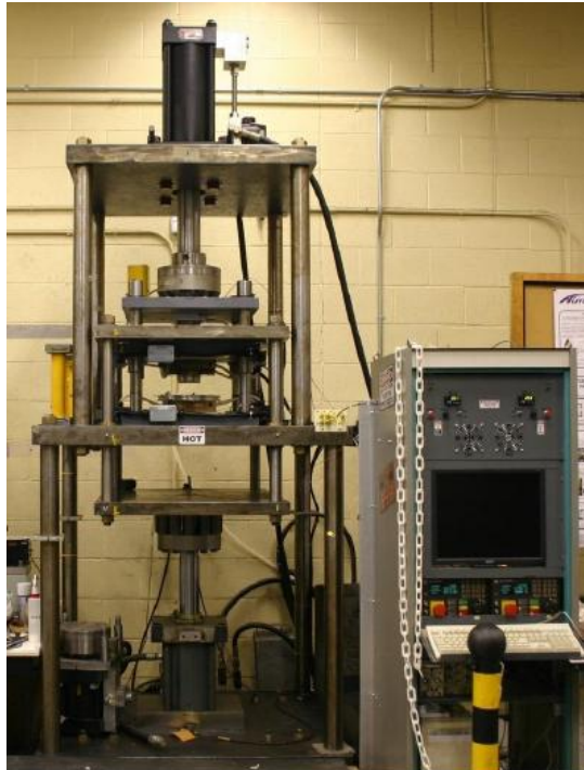
Figure 2.1: Experimental Setup; Hydraulic Press (left), computer control rack (right).
