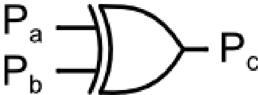
Figure 2.6: Simple circuit implementation of a 2-input parity-check node.
