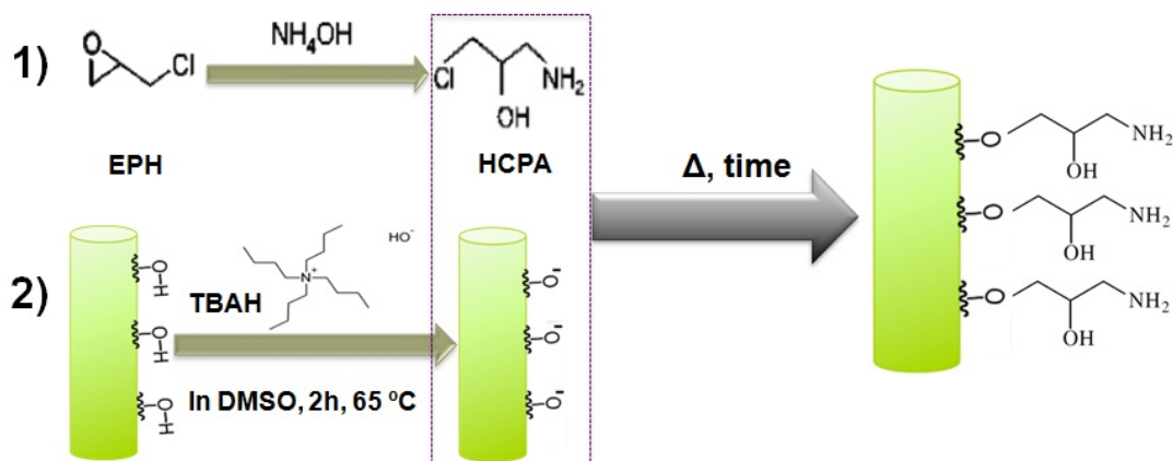
Figure 3.1: Two-step amine functionalization of CNC.
