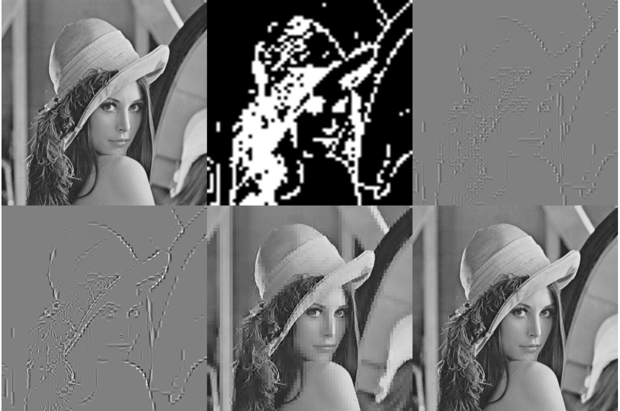
Figure 4.10: Multiresolution decoded images (MDI) for 512 \times 512 Lena (when d = 42 dB in PSNR). Top-left: Original image; Top-middle: MDI1-up-sampled OBF image with a scale factor of 8 (Rate: 0.007 bpp), by MCL1 only; Top-right: MDI2-decoded OTF image (Rate: 0.081 bpp), by up to MCL2; Bottom-left: MDI3-decoded outlier image (Rate: 0.159 bpp), by up to MCL3; Bottom-middle: MDI4-decoded outlier image with DC (Rate: 0.704 bpp), by up to MCL4; Bottom-right: MDI5-fully decoded image (Rate: 1.294 bpp), by up to MCL5.
