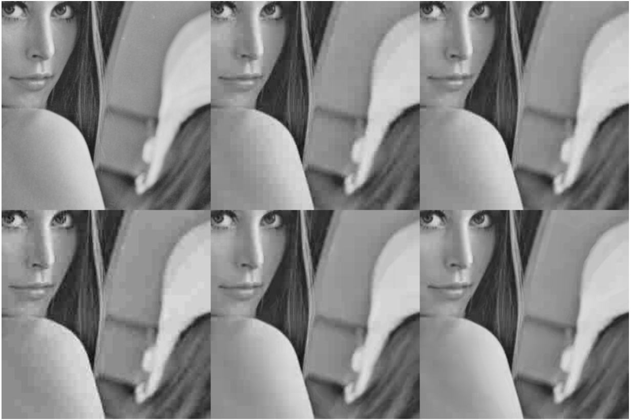
Figure 4.13: Subjective image quality comparison for 512 \times 512 Lena coded at 0.26 bpp. Top-left: original image (SSIM: 1, PSNR: inf dB); Top-middle: ECEB (SSIM: 0.942, PSNR: 33.32 dB); Top-right: the proposed (SSIM: 0.953, PSNR: 33.39 dB); Bottom-left: JPEG (SSIM: 0.931, PSNR: 31.90 dB); Bottom-middle: H.264/AVC (SSIM: 0.952, PSNR: 34.10 dB); Bottom-right: HEVC (SSIM: 0.959, PSNR: 34.84 dB)
