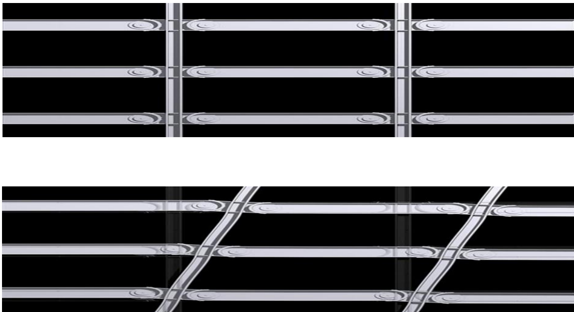
Figure 52: Pin-fuse joint behaviour during and after the earthquake shock (Skidmore, Owings, & Merrill, 2009)
