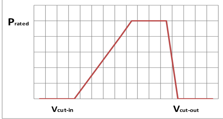
Figure 3.6: Wind Turbine Power Curve
