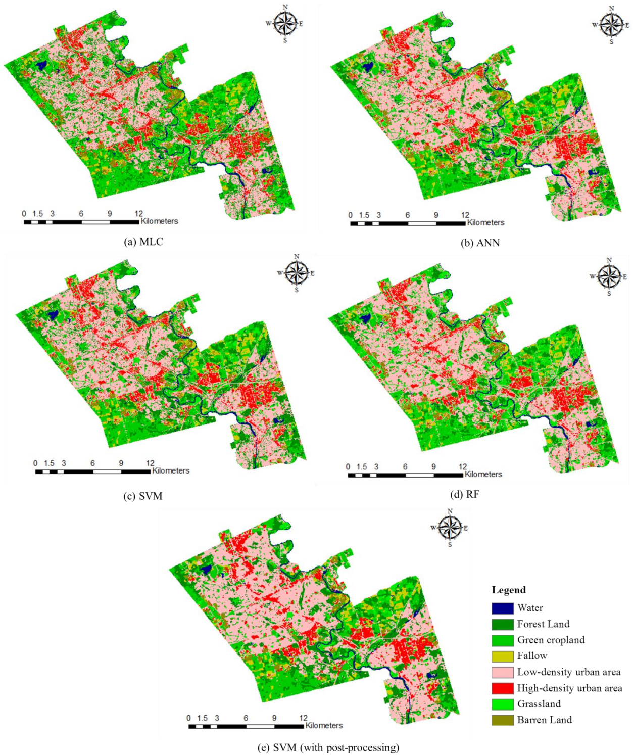
Figure 5.1 Classification maps of 2006 generated by (a) MLC, (b) ANN, (c) SVM, (d) RF, and (e) SVM with post-classification processing
