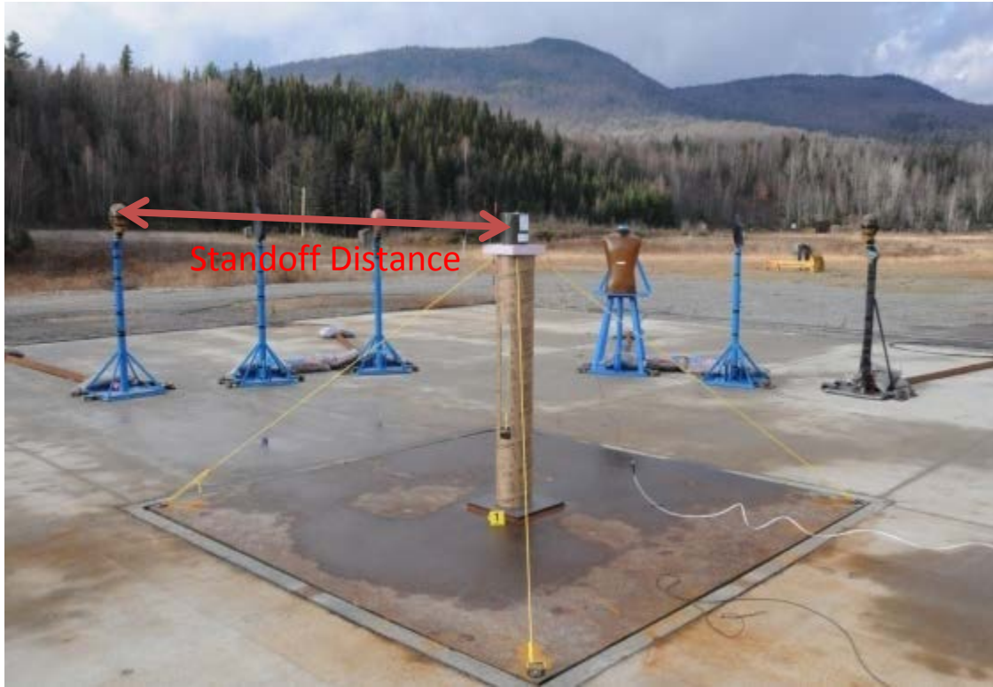
Figure 2-3 – Standoff distance between an explosive charge and target [Adapted from Ouellet et al., 2012].
