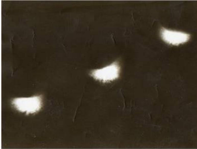
Figure 4.5a: (Above). X-ray radiograph of the base of 2 ml microfuge tube after centrifugation, looking at the material pellets after decalcification over a period of 1-3 days at 37 °C (left-right).
