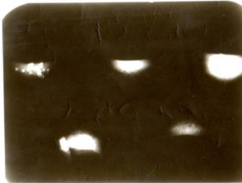
Figure 4.6a: (Above) X-ray radiograph of the base of 2 ml microfuge tube, after centrifugation, looking at the material pellets after decalcification over a period of 1-5 days at 56°C (left-right/top-bottom).
