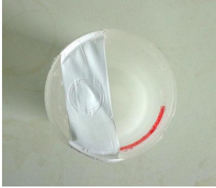
Figure 4.3 – Teflon® tape enclosing the acidified filter disc and laid across the top of the diffusion container.
