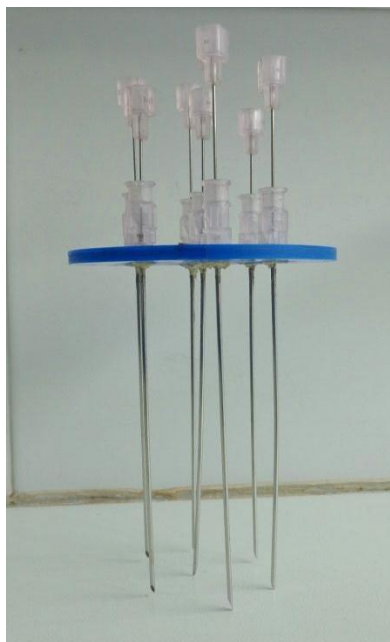
Figure 4.1 – Needles of the multi-injection system with wires partially inserted.
