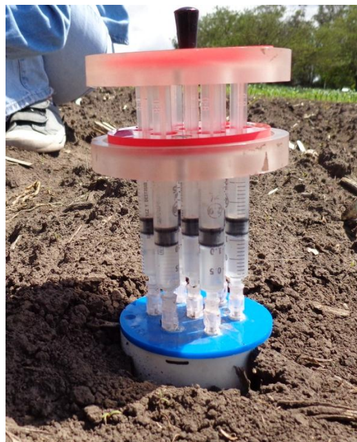
Figure 4.2 – Multi-injection system containing the (^{15}\text{NH}_4^+)_2\text{SO}_4 solution immediately prior to injection.
