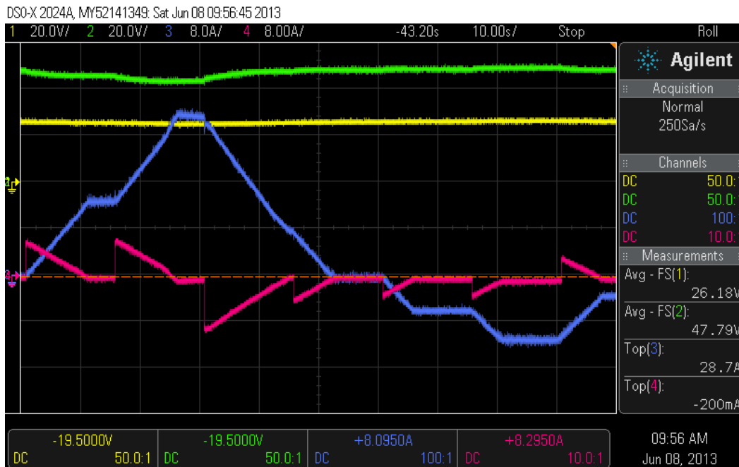
Figure 4-13 Experiment results of BU discharging current and UC discharging current under hard testing condition: BU discharging current (blue); UC discharging current (pink); BU terminal voltage (yellow); DC-bus voltage (green)
