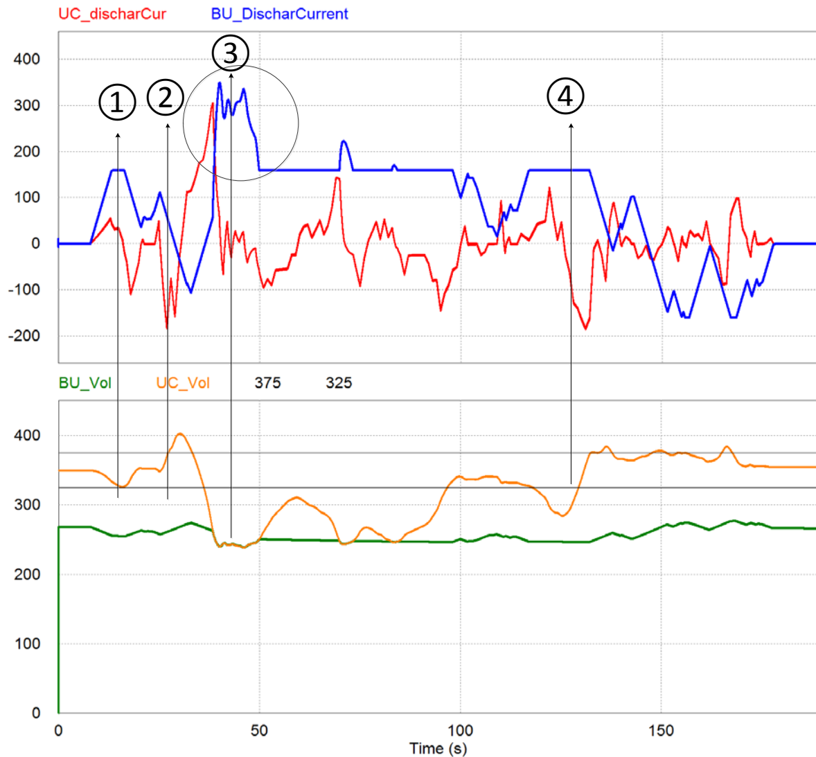
Figure 3-21 BU discharging current, UC discharging current, BU terminal voltage, and UC terminal voltage from PISM simulation for Tesla Model S on the 189s of the UDDS drive cycle
