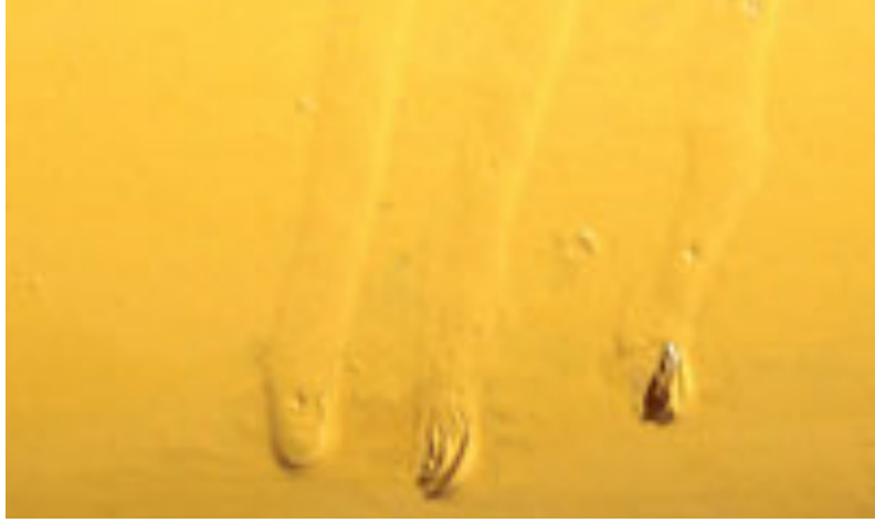
Figure 5.5: The phenomenon of the flow of a thin paint over a wet painted wall.
