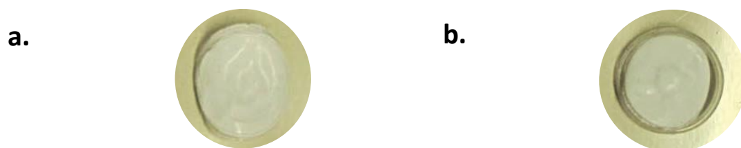
Figure 55. Celgard® separators recovered from coin cells a. half-discharged and b. fully discharged.
