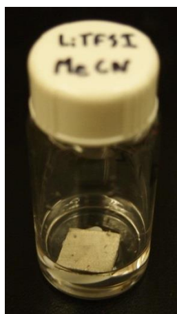
Figure 42. Metallic lithium immersed in a (ACN)_2:LiTFSI solution for one month.
