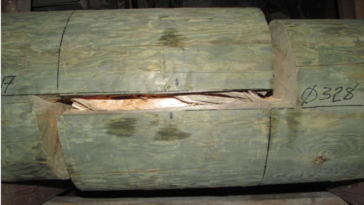
Figure 3.5 Failed specimen with one failure plane perpendicular to the notches
