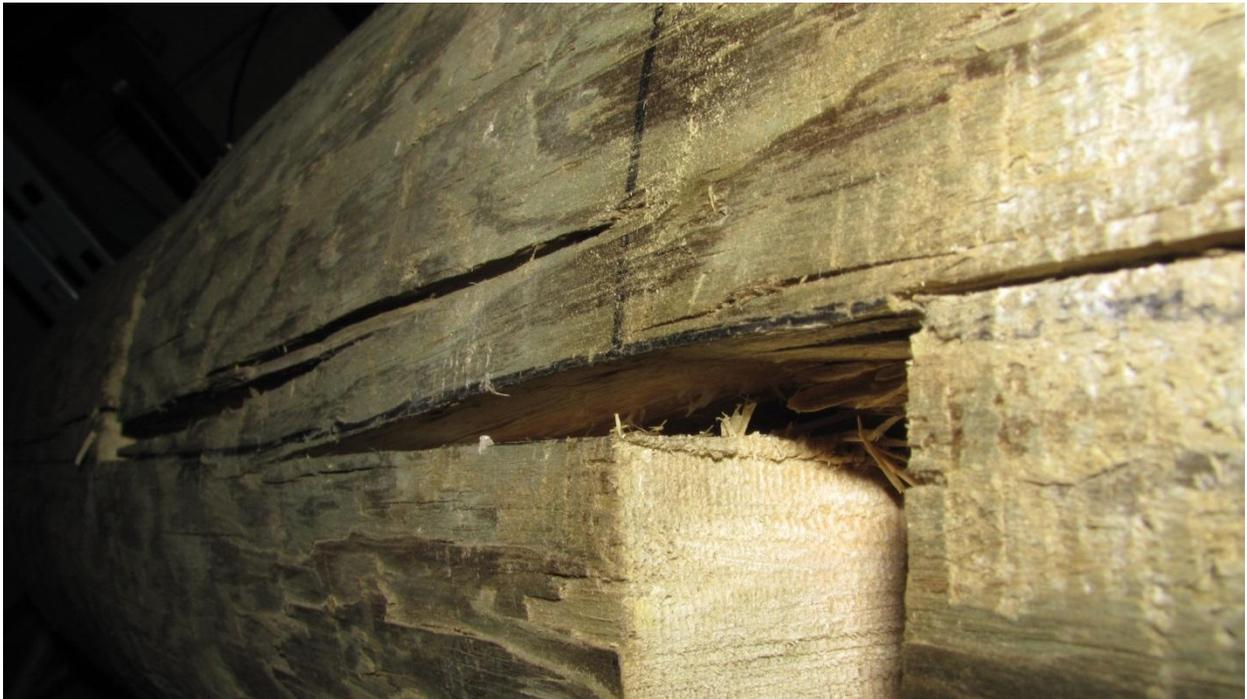
Figure 3.7 Failed specimen with strut and two separate failure planes
