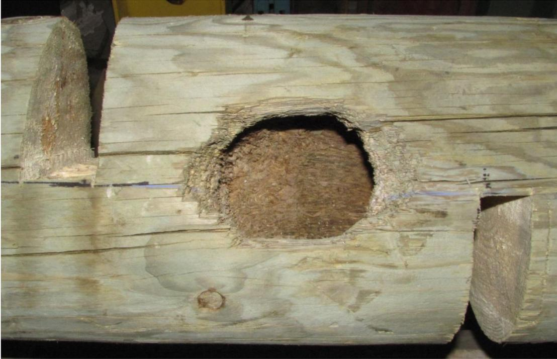
Figure 3.9 Untested specimen with woodpecker damage
