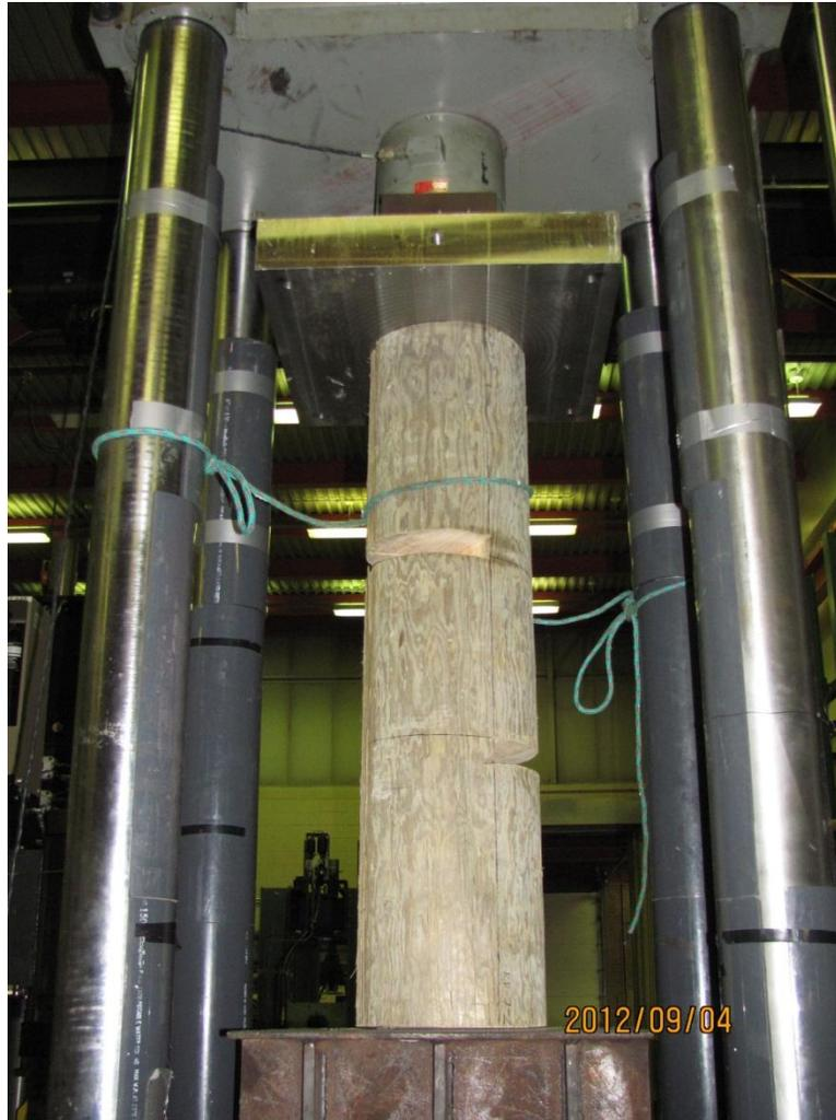
Figure 3.4 MTS 311 test frame with a specimen ready to be tested
