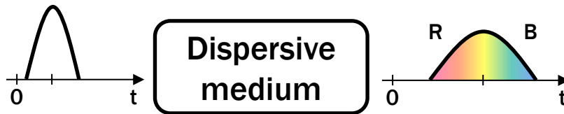
Figure 2.4: A dispersive medium broadens a pulse of light. When a pulse of light propagates through a dispersive medium, each frequency component travels at a different speed, causing the pulse to broaden in time. The shorter wavelengths (B) lag behind the longer wavelengths (R) in this example.
