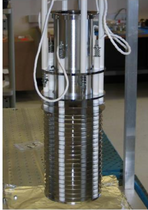
Figure 3-7 A photograph of a real TOF spectrometer being used at ALLS laser facility
