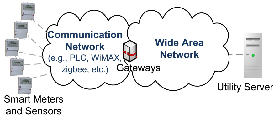
Figure 1.2: Smart Metering Network Architecture
