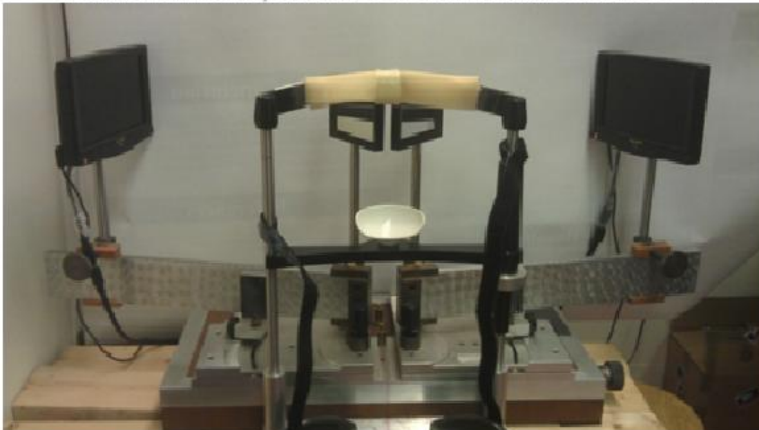
M1 and M2 - front surface mirrors, S1 and S2 - LCD monitors, L and R - left and right eye and its tracker. Mirror to eye distance - 10 cm and Mirror to screen distance 30 cm.
