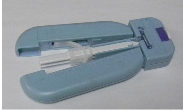
Figure 4-2 Fiber strippers for polymer removal
