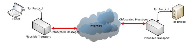
Figure 1.2: Pluggable transport overview: Messages are reformated or embedded in a cover protocol to bypass detection tools.
