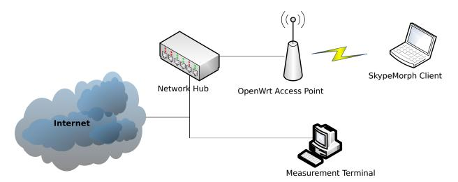
Figure 7.2: Our network setup for experimental run of SkypeMorph on OpenWrt. A node is connected through wireless to the OpenWrt router and a hub is used to intercept the outgoing packets to create a trace.
