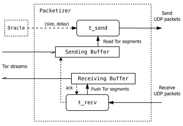
Figure 6.4: Structure of the packetizer.
