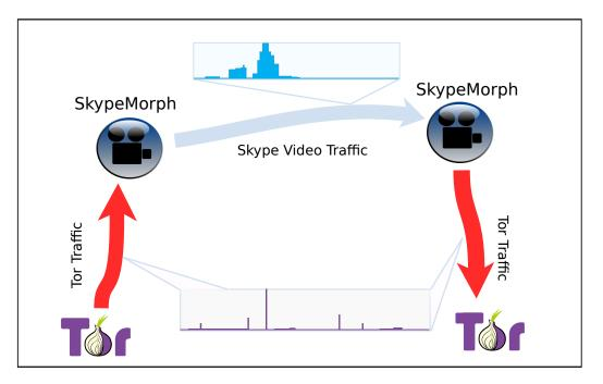
Figure 5.1: High-level overview of the SkypeMorph Architecture. The histograms show the distribution of packet sizes in Tor (at the bottom) and Skype video (at the top).
