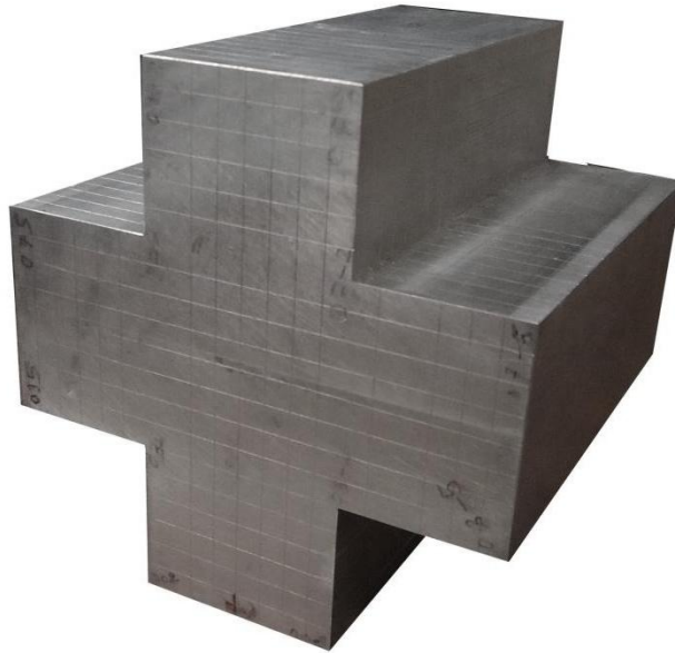
Figure 4-5 Reference object used for calibration of 8 cameras
