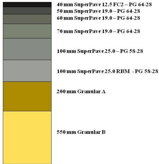
Figure 3-2: Cross-Section of Perpetual Pavement with RBM
