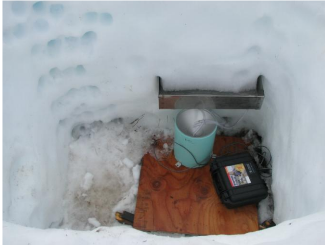
Figure 3.2 lysimeter and tipping bucket in snow pit #1
