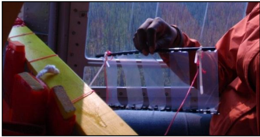
Step 1: Assemble the sampler in the helicopter. This is made easy by propping the sampler stick so that the units can hang down freely and placing the anchor in the foot area.
