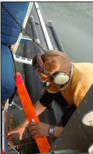
Step 3: Field technician has released the anchor into the water and is holding onto the sampler stick with the other until the anchor has reached the bottom.
