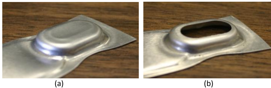
Figure 6.2 Current heat exchanger plate component: (a) as formed and (b) after piercing the coolant channel.
