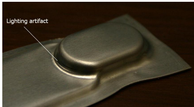
Figure 6.8 Forming using Teflon sheet as lubricant, 6.72 kN clamping force, heated dies at 300°C and cold punch at 15°C
