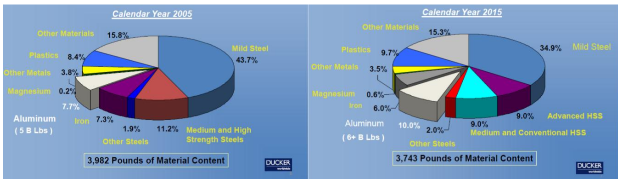
Figure 1.3 Recent (left) and expected (right) material content of light weight North American vehicles [Ducker Worldwide Institute]
