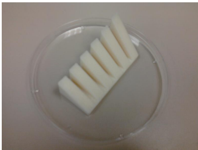
Figure 32 - Schematic showing the deposition process for substrates mounted on an incline
