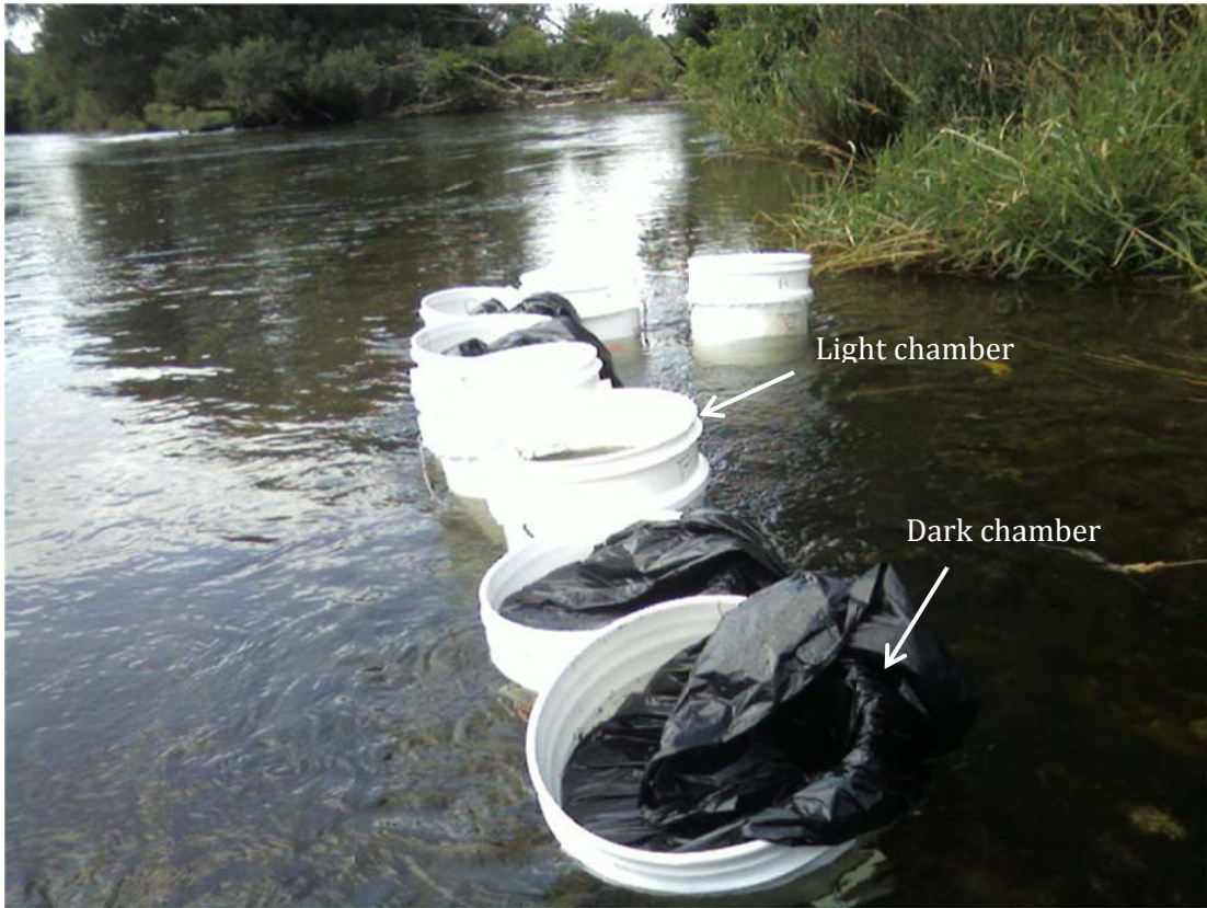
Figure 5.2 In-situ chamber incubation setup in the Speed River showing light and dark chambers.
