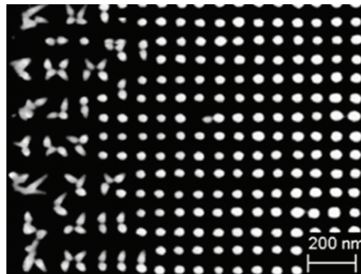
Figure 2.9: Top view of the nanowires with length of 400 \text{ nm} as the average diameter is increased gradually from 25 \text{ nm} to 50 \text{ nm} . Nanowires with diameters greater than 34 \text{ nm} are vertical whereas the ones with diameter below 32 \text{ nm} bunch. An abrupt transition is observed [1].
