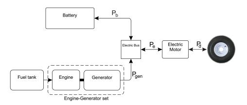
Figure 2.1: Schematic of a series HEV
