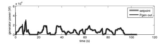
Figure 4.8: Tracking performance of the lower level controllers of the engine-generator set
