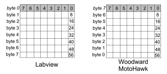
Figure 4.3: Different byte allocation methods in CAN data frame
