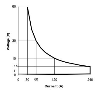
Figure 5.7: The operating curve for the Sorensen SLH 1800-60-240 electric load, [54]
