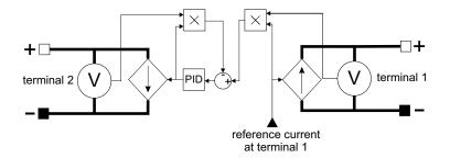
Figure 3.2: Schematic of the DC/DC converter
