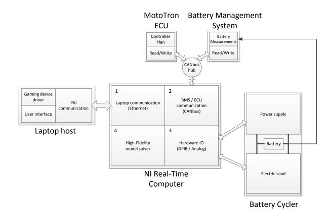
Figure 4.2: Schematic of the HIL setup
