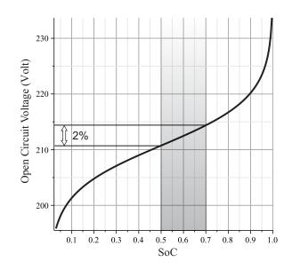
Figure 2.3: Simulation results for the open circuit voltage versus the state of charge in a NiMH battery pack [40]
