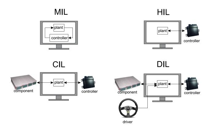
Figure 1.2: Schematic of the different simulation setups
