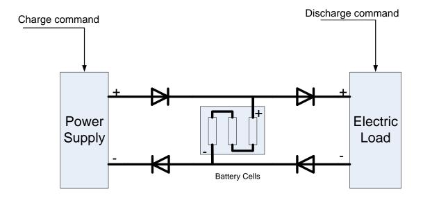
Figure 5.3: The schematic of the battery cycler
