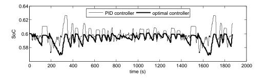
Figure 3.7: Comparison of SoC trajectories for the FTP75 drive cycle for the two controllers
