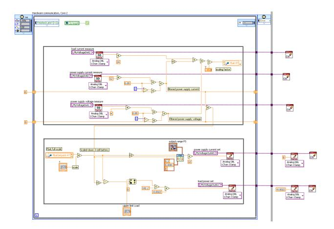
Figure H.3: The battery cycler control loop, core 3
