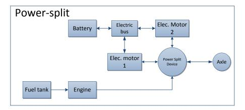
Figure 1.1: Different configurations in hybrid electric powertrains
