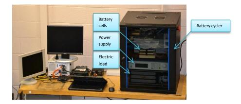
Figure 5.2: The component–in-the-loop setup
