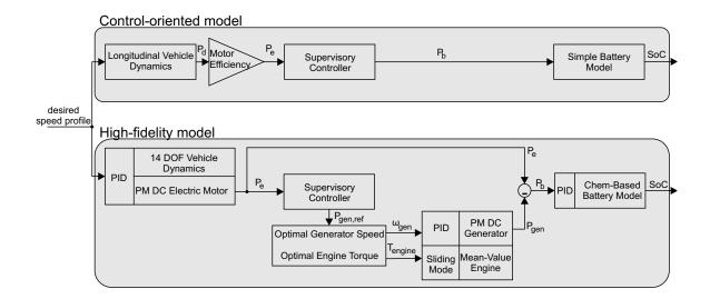
Figure 3.5: Simplified schematic of the simulations to validate controller-oriented model
