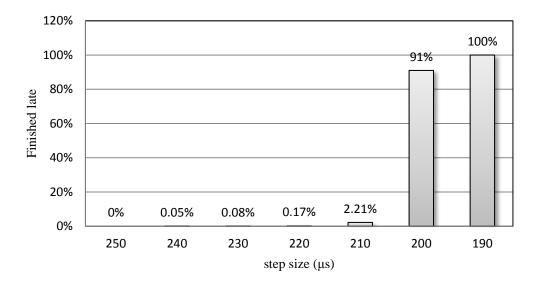
Figure 4.6: Number of iterations finished late for different step sizes
