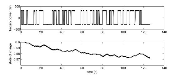
Figure 5.15: The excitation input and the resulting output of battery
