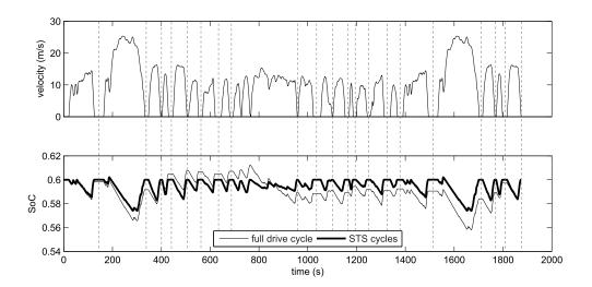
Figure 2.7: State trajectory when considering the full drive cycle, and when considering STS cycles
