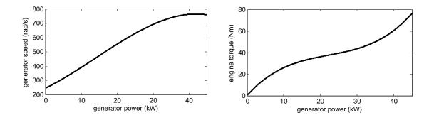
Figure 3.4: Optimal engine torque and generator speed versus generator output power
