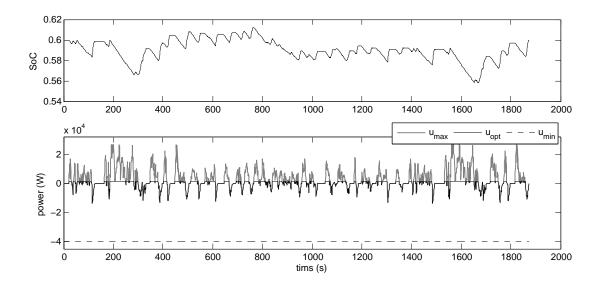
Figure 2.10: The optimal SoC and control trajectories for the FTP75 drive cycle found using the PMP solution
