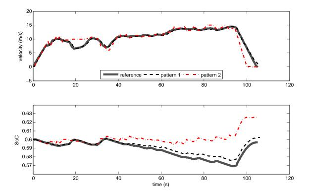
Figure 6.2: Velocity profile and state of charge trajectory for different driving patterns
