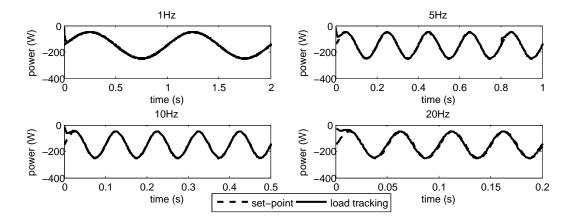
Figure 5.12: Tracking performance of the electric load
