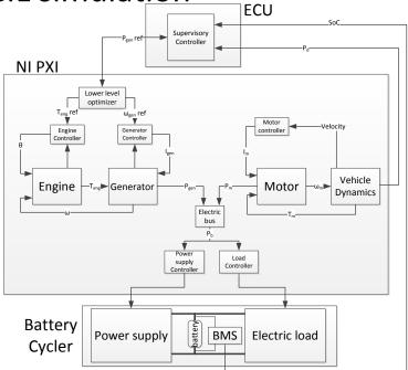
Figure 5.1: HIL and CIL simulation setup
