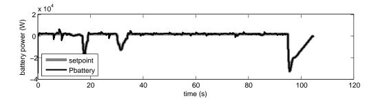
Figure 4.9: The comparison of optimal battery power, defined by the controller, and the real battery power
