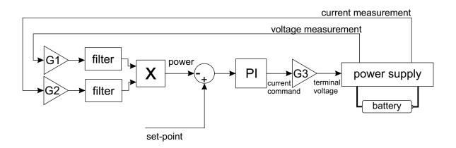
Figure 5.9: The control loop for power supply
