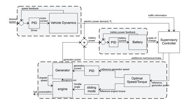
Figure 3.3: Schematic of the causal HEV model used in the control loop
