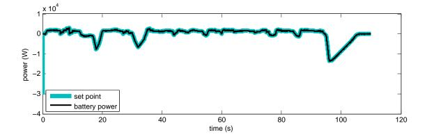
Figure 5.17: Tracking performance of the battery cycler
