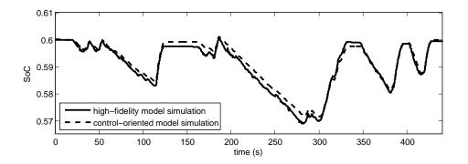
Figure 3.6: State of charge trajectory for the first 440s of FTP75 drive cycle
