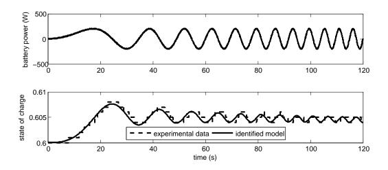
Figure 5.16: Comparison of the state of charge trajectories between the identified model and the physical battery
