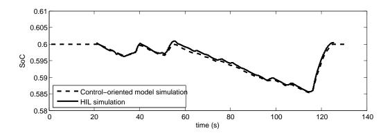
Figure 4.7: The comparison of SoC between control-oriented model simulation and HIL simulation
