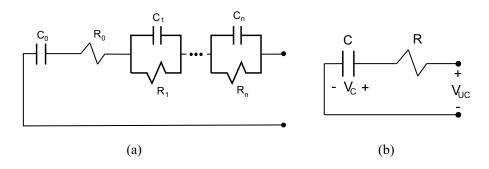
Figure 2.9: Ultra-capacitor circuit model
