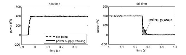
Figure 5.13: Rise time and fall time of the power supply
