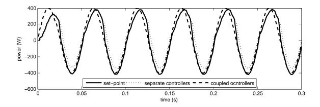
Figure 5.14: Improvement in tracking performance of the battery cycler at 20Hz
