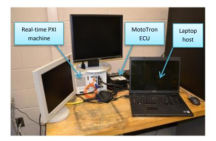
Figure 4.1: The HIL simulation setup developed
