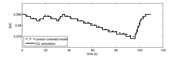
Figure 5.18: CIL simulation results for the state of charge trajectory for the first part of the FTP75 drive cycle
