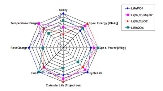
Figure 5.4: Comparison of different technologies for Li-ion battery [51]
