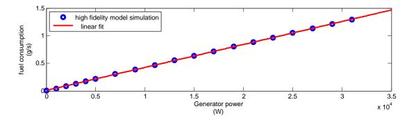
Figure 2.4: Simulation results for the minimal fuel consumption rate versus generator power
