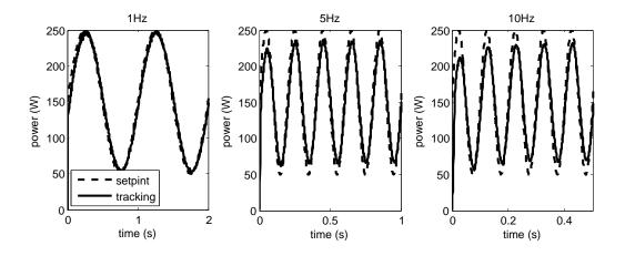
Figure 5.10: Tracking performance of the power supply
