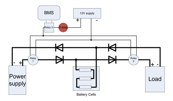
Figure 5.8: Schematic of the electrical circuits
