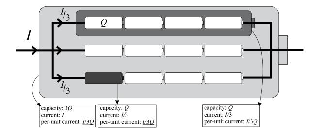
Figure 5.5: Per-unit current for different cells in a battery pack
