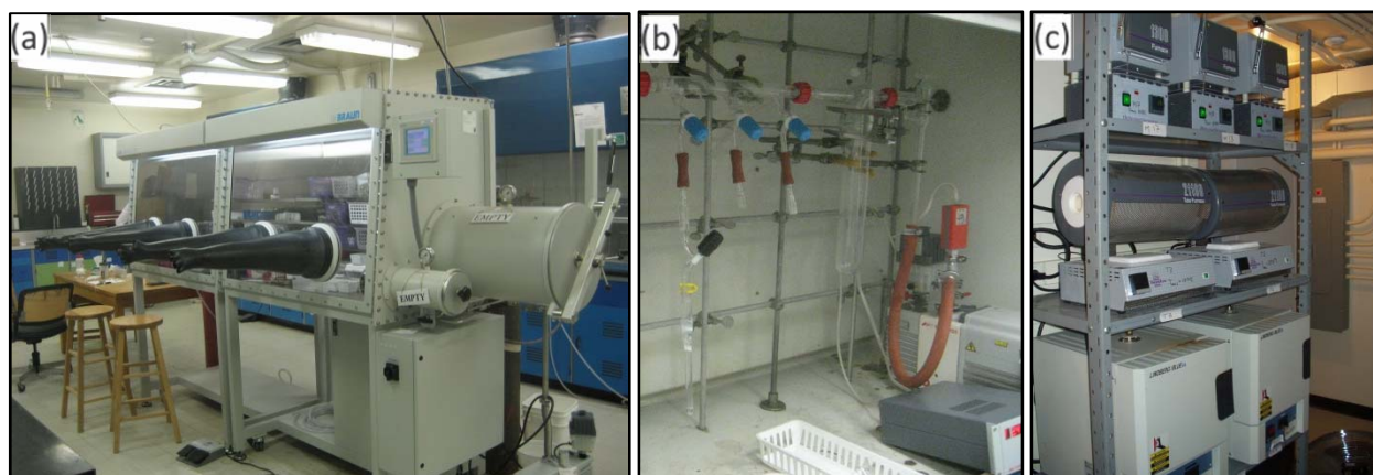
Figure 3.1 (a) Argon-filled glove box (b) Vacuum line and quartz sample tube (c) Manual (top), tube (middle), and programmable furnace (bottom).
