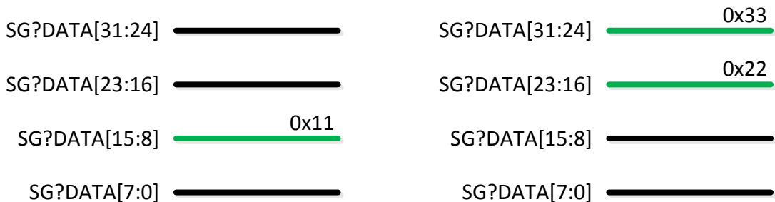
(a) 8-bit transfer of 0x11 to a memory address ending in 0x1 (b) 16-bit transfer of 0x3322 to a memory address ending in 0x2
