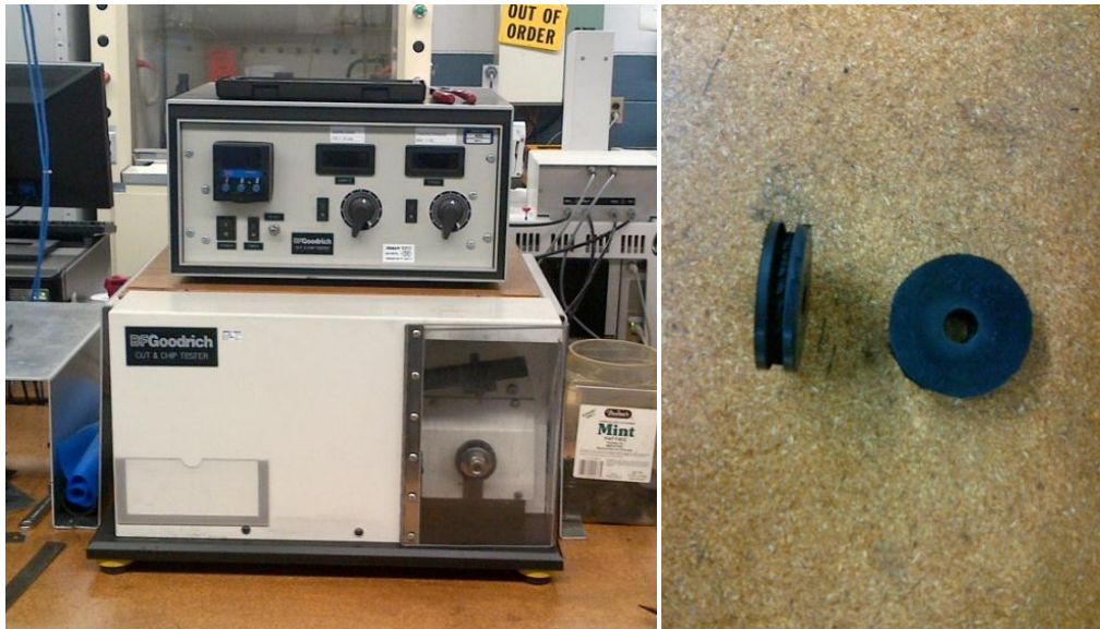
Figure 3.11: BF Goodrich cut and chip tester (left) and cut and chip specimen after test (right)
