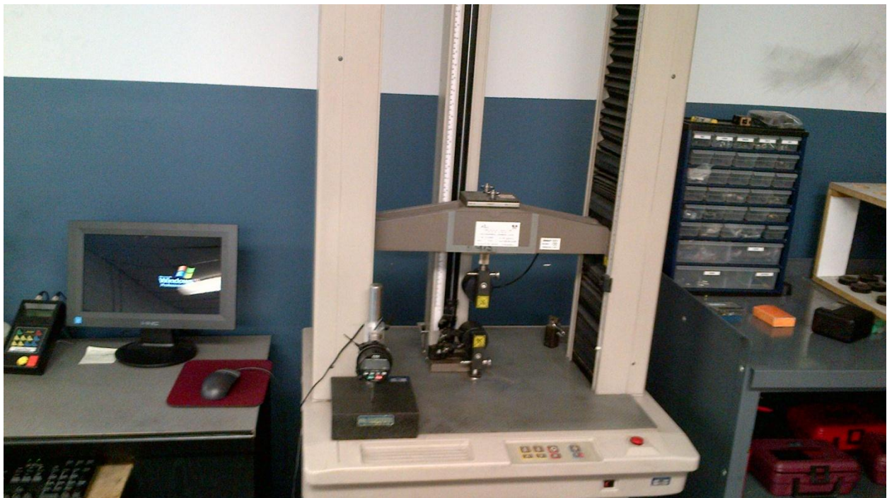
Fig 3.6: Tensile testing machine (Monsanto model 500 located in Airboss)
